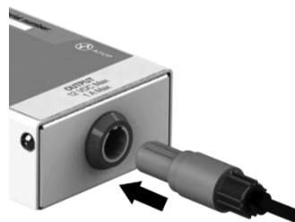
Connecting the cable to the control unit.
